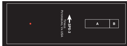
Test No. 6, SPS-3 Heterophorias Muscle imbalance-vertical and lateral is tested at predetermined pass/fail levels. This test is administered first at far, then at near.
