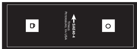
Test No. 4, SAE-40-4 Right and Left Eye 20/40 Acuity Different Symbol Each Eye. Also available 20/30 Acuity.
