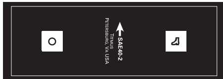
Test No. 2, SAE-40-2 Right and Left Eye 20/40 Acuity Different Symbol Each Eye. Also available 20/30 Acuity.
