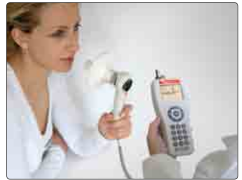
Display: Black and white LCD display (320x240 pixels) with real time monitoring of test performance, plus encouragement features for children and non-cooperative patients;
