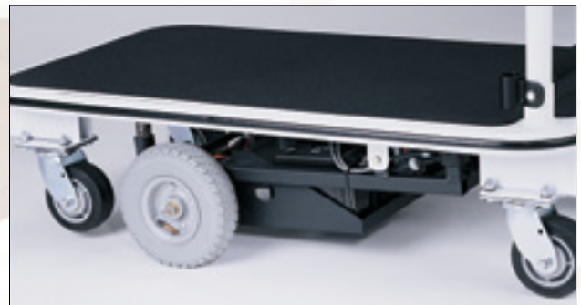
Center wheel drive system with Flat-free tires
